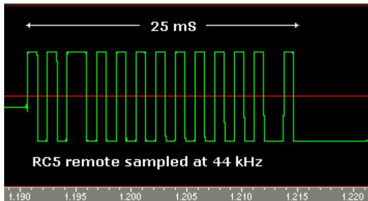
This is what I've got from an RC5 remote placed at 15 cm from a BPW41 photodiode and a 100 kohm resistor. The original high frequency modulation is cut out by the sound card input filter, leaving a clean, intelligible waveform. Perfect!
