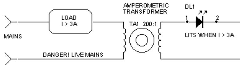
Replace the LED with an optocoupler and connect it to the PC serial or parallel port to monitor when an appliance or an industrial equipment is working (a square wave is output)
