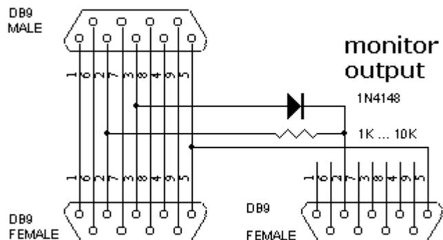
pulls the monitor output to the RS232 rest potential (negative) when no data is transmitted.
