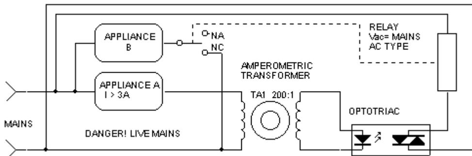
I use this priority switch to automatically remove power from appliance B when A is powered on. That is, A takes precedence over B, and the maximum power consumption is never exceeded.
