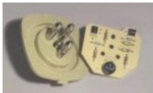
*The whole circuit is placed inside the phone plug. The LED is visible drilling a hole on the back shell. Now I know why italian phone plugs are so large!!!*
